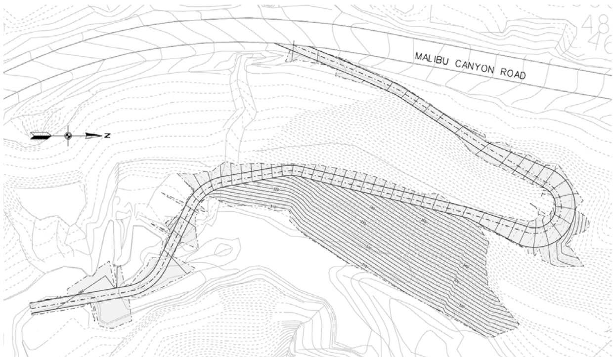
Figure 4.2-8 Reconstructed Invert Access Ramp
