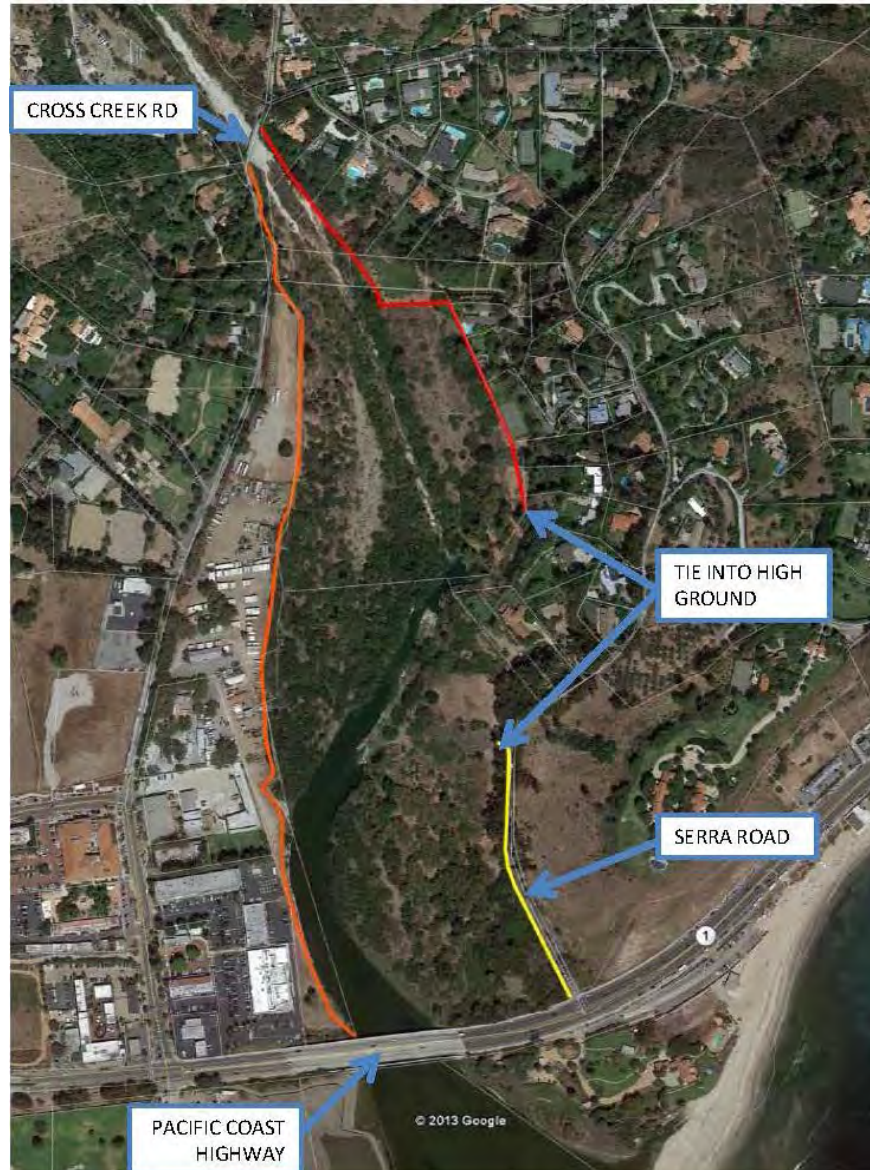
Figure 1.3-1 Downstream Floodwalls. Downstream Mitigation Layout
