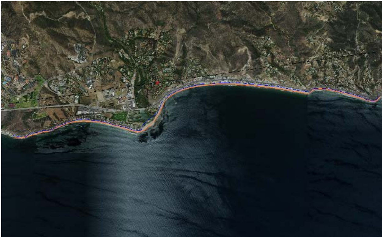
25 26 Figure 4.3-1: GenCade model domain and initial conditions. Black line indicates the cells and 27 reference line, red circle shows offshore wave input location, blue line is the seawall/revetment and 28 orange line is the shoreline
