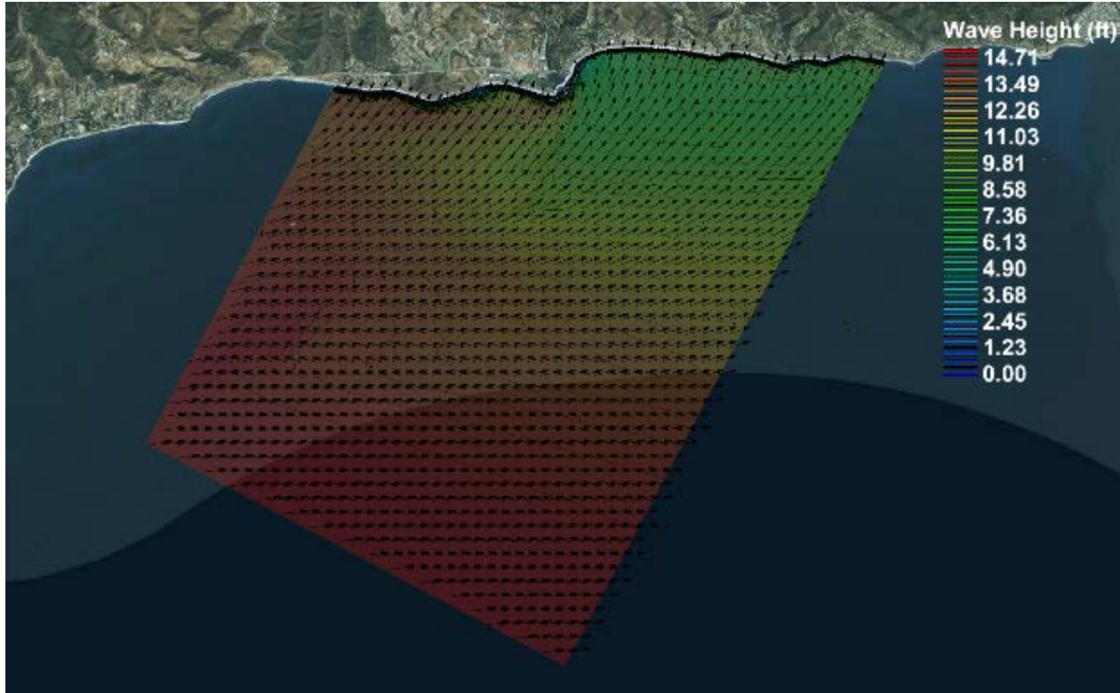
1 2 Figure 4.1-3: Maximum recorded wave height conditions at project location ( H_s=14.75\text{ft} , T_p=14\text{s} , 3 D_p=262^\circ )
