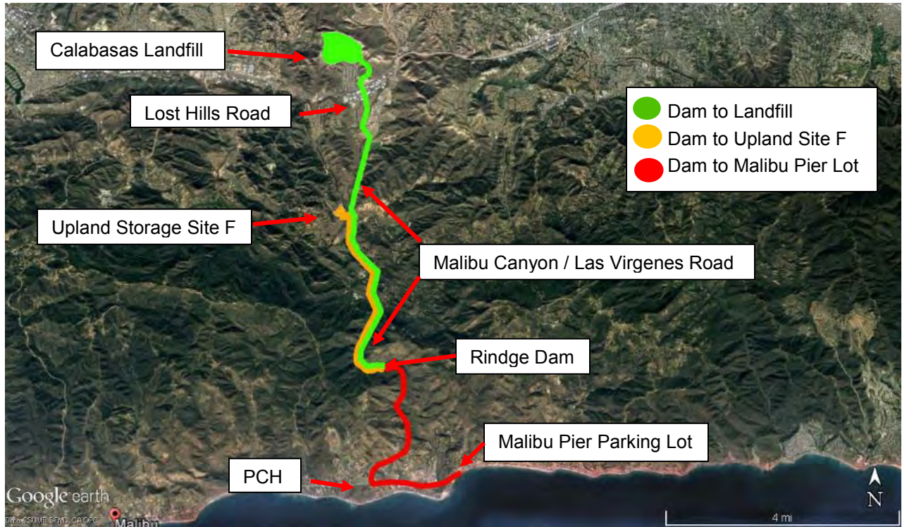
Figure 4.4-8 - Trucking Routes for Rindge Dam Impounded Sediment (Alts 2a1, 2b1, 2c1, 2d1)
