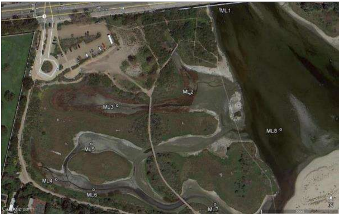
Figure 15. Map of pre-restoration water quality monitoring stations. ML2 and ML6 are the locations of the pre-restoration permanently-deployed YSI data sondes.
