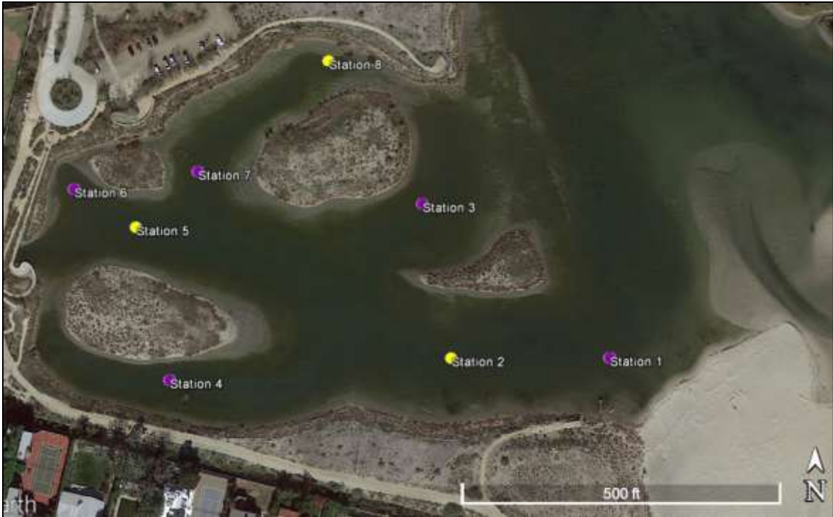
Figure 14. Map of post-restoration vertical profile, SAV/algae, surface and bottom water nutrient, and sediment survey stations. Stations 2, 5, and 8 are the locations of the three permanently-deployed Hydrolab data sondes (in yellow).
